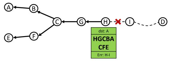
The Route Error is divided into multiple packets at the branch point.
